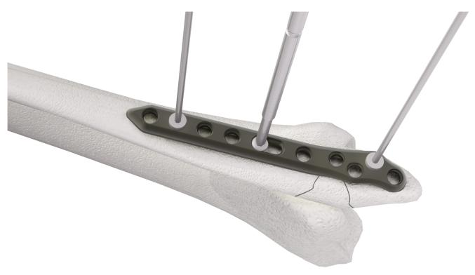
Then using the spiral drill, D=2.7mm, L=100mm, AO Connector (61273-100) to drill through
