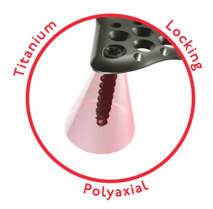
When a locking screw is inserted, it forms threads into the plate. There is no cutting and thus no debris created. Each locking screw can be locked at a free placement within a cone of angulation up to  $\pm$  15°, and can be re-positioned up to three times.
