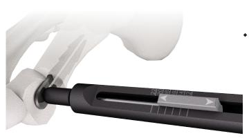
When measuring directly on the plate, read off the required screw length on the **front** edge of the sliding handle.
